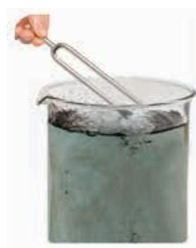
Tip of a vibrating tuning fork produces disturbances on water surface.
