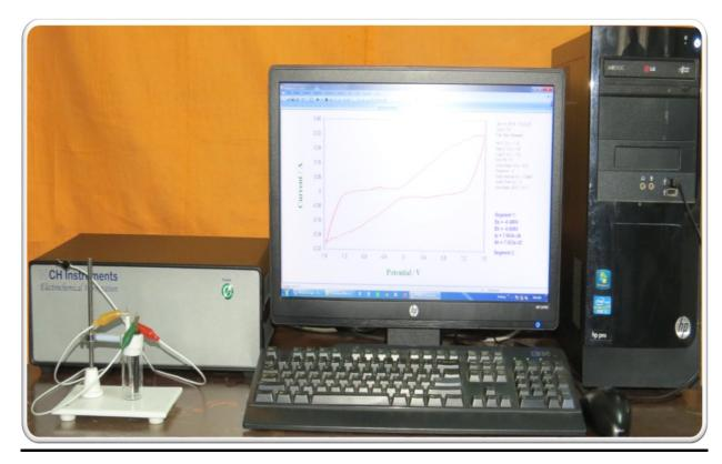
The model 600E series instrument is a computerized general purpose potentiostat / galvanostat. The potential control range is ±10V and the current range is ±250mA. The instrument is capable of measuring current down to picoamperes.
