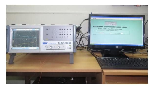
Wayne Kerr 6500B Precision Impedance Analyzers provide precise and fast testing of components at frequencies upto 120 MHz. The instrument can be used for many different tasks and applications including passive component design, dielectric material characterisation and manufacturing test.
