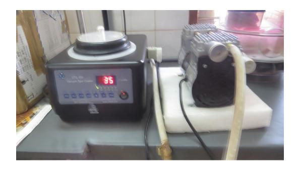
VTC-100A is CE certified compact spin coater with vacuum chucks designed for easy and quick coating via sol-gel for wafers up to 4". The spinning speed is variable from 500-8000 rpm with two programmable segments.
