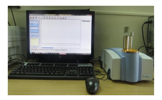
Bruker Alpha Spectrometer is an easy to use FT-IR sampling method that is suitable for both solids and liquids and does not require any sample preparation. The Eco ATR is a single reflection ATR sampling module with a very high performance ratio. It is equipped with a versatile high throughput ZnSe ATR crystal for the analysis of powders, solids, pastes and liquids.
